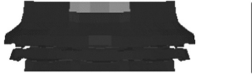
Fig. 25.6 Comparisons of crash results – thin-walled octagonal tube model: deformed configurations
